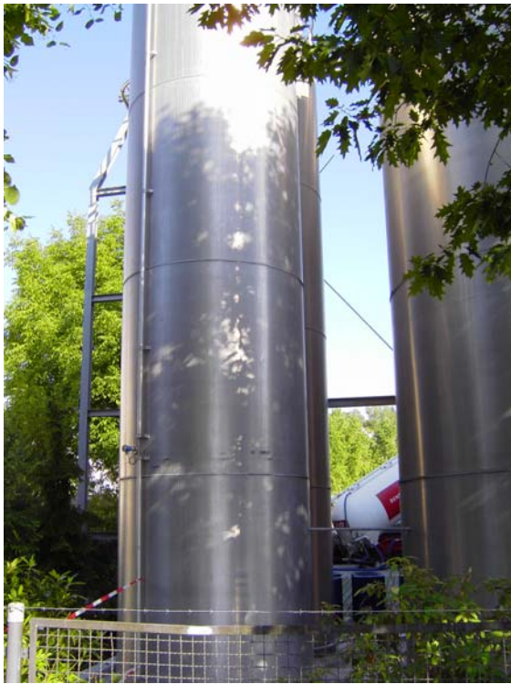
Soliphant T - FTM20 Low Level detection in a 33 ft high toothpaste powder to trigger the re-order process of the material
